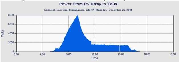
Having this feedback from the sites in the field allows Apollo Solar to close the loop with our system designs and to verify the operation of every part of the energy equipment at the sites.
