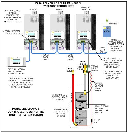
Figure 1: Network Wiring Diagram
