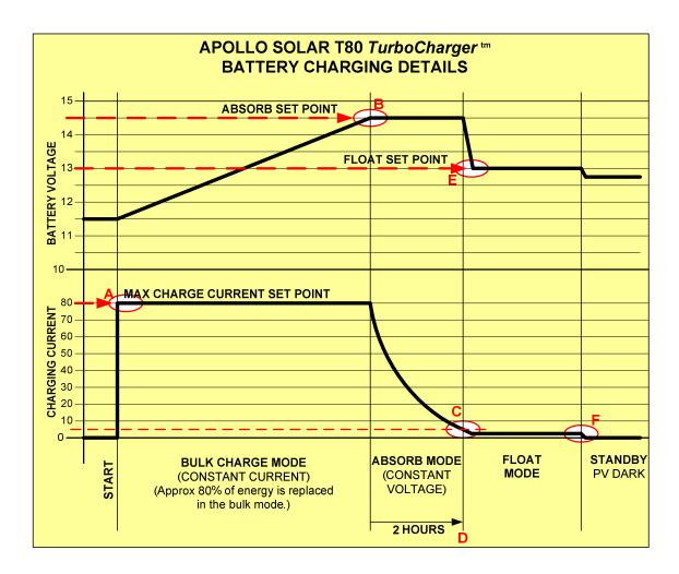
**Bulk:** In the Bulk Mode the Controller is trying to get the battery voltage up to the Absorb Voltage Setting (B). It will use all the power it can get from the panels limited only by the Maximum Charge setting (A). When the Absorb Voltage is reached on the batteries, the charger switches into Absorb Mode.
