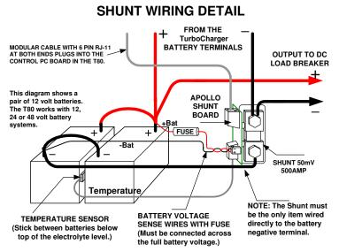
Voltage Sense Wire Installation— Push the white connector on the wire assembly onto the white connector on the Apollo Shunt circuit board after connecting the red wire to a battery positive buss and the black wire to a battery negative buss within the DC load center. Be sure to observe correct polarity when installing voltage sense wires or damage will result. Note: Fuse on positive battery terminal (1/2A 5mm x 20mm fuse).
