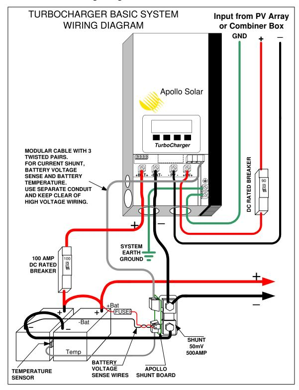
The drawing above shows a schematic of the TurboCharger™ installed in a battery system. Remember all circuit protection devices must be installed inside appropriately rated UL recognized enclosures.
