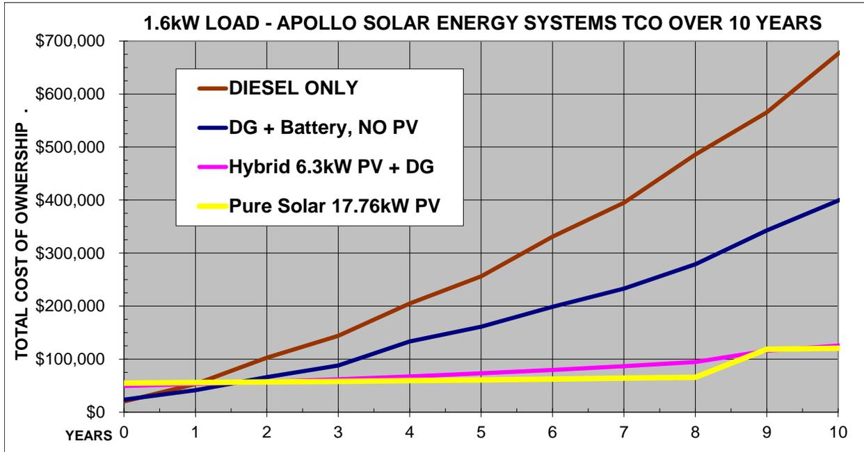
**CHART OF TOTAL COST OF OWNERSHIP** above shows both the CAPEX and OPEX of base case DG only, and 3 plateaus of improvements: DG+Batt, Hybrid PV/DG and Pure Solar over 10 years.
