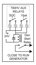
The Apollo Solar PVT Gen4 Mini Cabinet uses a single T80HV Charge Controller. Each T80HV is equipped with 2 Auxiliary Relays which can used to switch on external items triggered by the parameters which are monitored internally by the T80HV. These parameters include the Battery State of Charge and the Battery Voltage.
