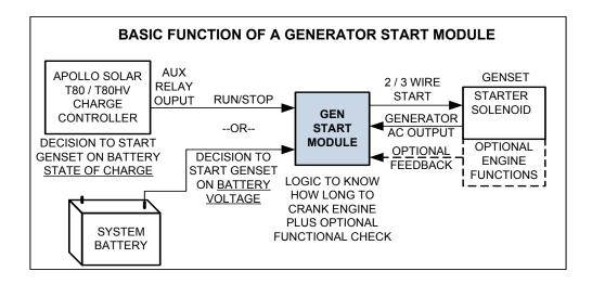
In the block diagram above, the Gen Start Module is the device that must be added to make the genset as smart as it has to be for automatic starting. The decision of when to start is still made by the Apollo Solar T80 or TSW True Sine Wave Inverter / Charger. The third party Gen Start Module is connected between the T80 AUX Relay contacts and the generator.
